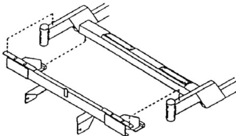
**ADJUSTMENT** - Loosen the four (4) nuts on the sides of the tray mounting brackets. Adjust the tine tray to locate the tine ends approximately 1/2" above the flat surface when in the free position and touching the flat surface when pushed back. Tighten four (4) nuts.
